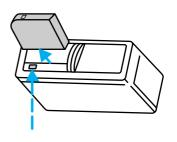
Make sure only one disc is inserted in each slot. Each disc must be inserted with the label surface upward. You may insert up to six CDs.
